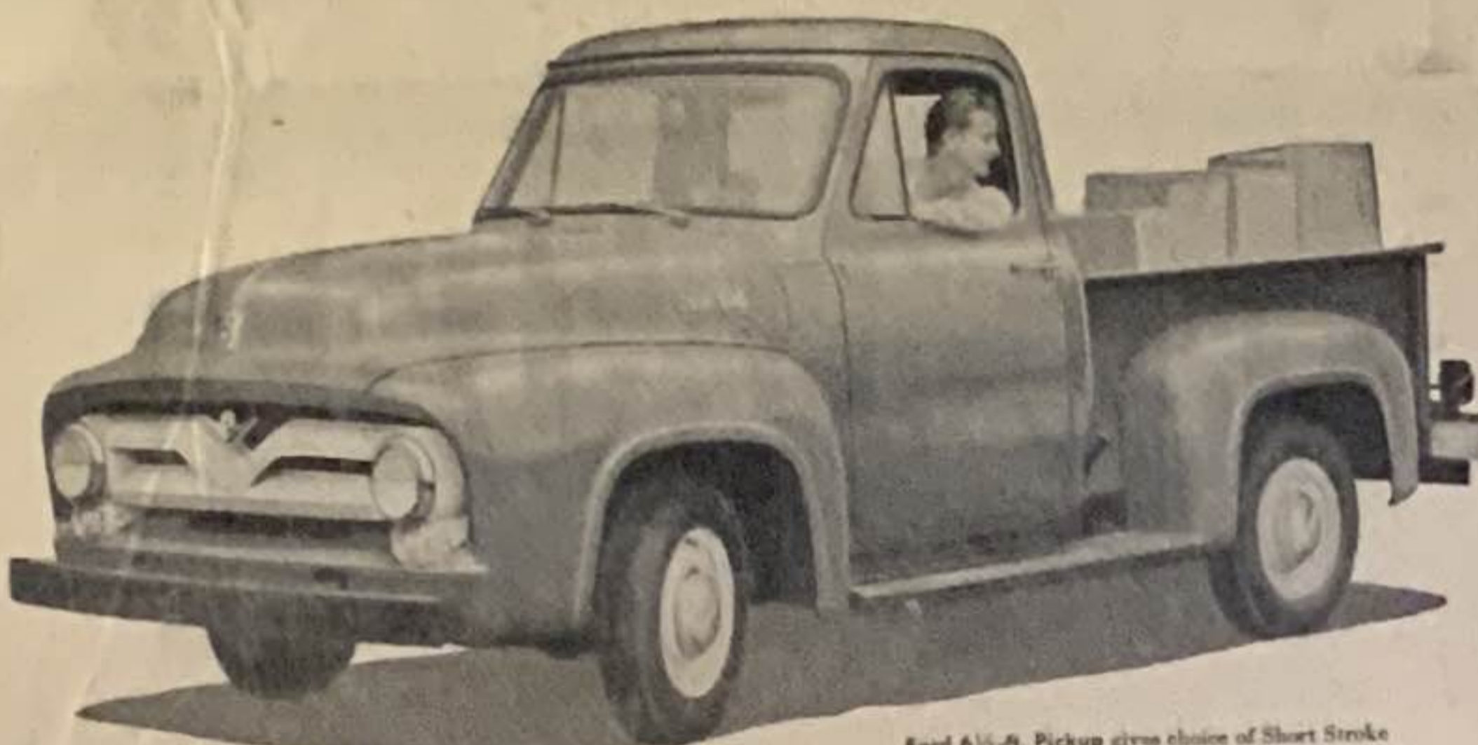
Ford 6 1/2-ton Pickup gives choice of Short Stroke 122-h.p. V-8 or Short Stroke 115-h.p. Six. Tabeless tires standard. Fordomatic Drive and Power Brakes available at low extra cost. GVW 5,900 lbs.
